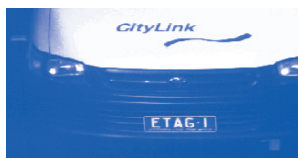
Figure 1: Digital image of LPN taken by infra red camera following exception (image reproduced here with consent of vehicle owner).
